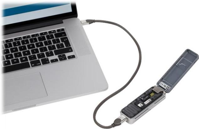
Figure 3: Oxford Nanopore Technologies MinION sequencer connected to the USB port of a laptop. Credit: Oxford Nanopore Technologies (<https://nanoporetech.com/about-us/for-the-media#image123634281&modal=image123634281>).
