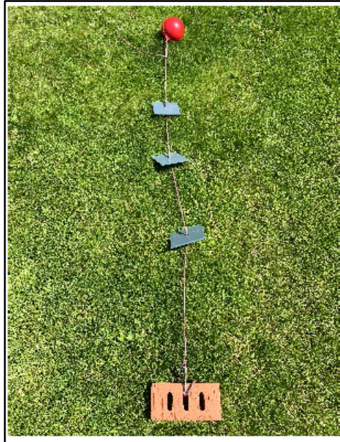
Figure 2.2. Settlement plates applied in each harbor.
