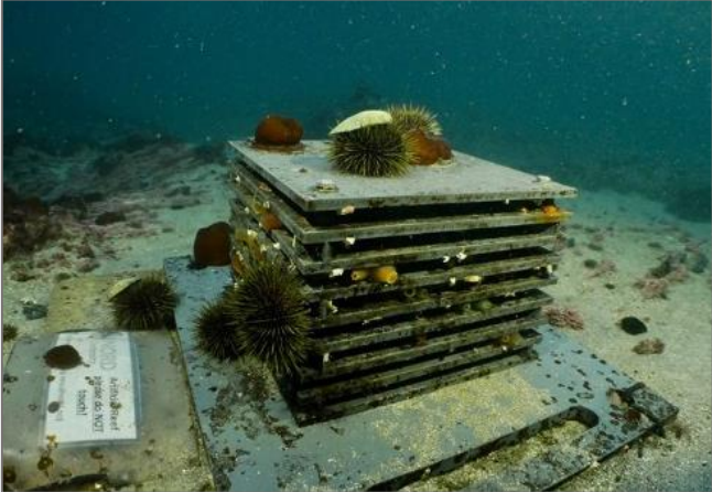
Autonomous Reef Monitoring Structures (ARMS)
